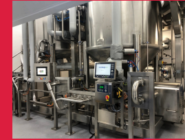
ADPRO VACUUM PROCESSING MIXER 50L TO 6000L CAPACITY
